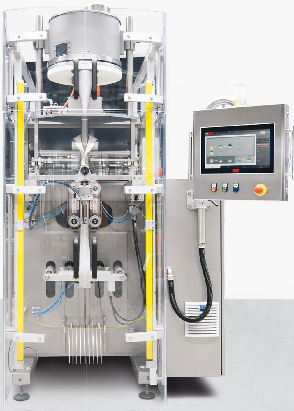
→ Vertical FFS machine fully automated thanks to the Vertical Form Fill and Seal StarterSET
