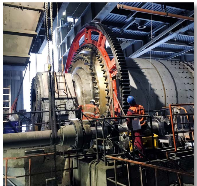
Figure 4: New girth gear made from ADI is only 300 mm wide (Photo: Cemex)
